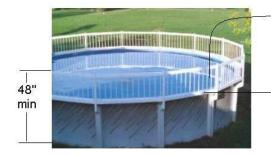
openings shall not allow the passage of a 4" sphere at any point within the 48" barrier
